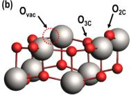
Fig. 2 The anatase  $TiO_2$  (001) surface with (a) the fully oxidized surface having one pair each of  $O_{2C}$  and  $O_{3C}$ , and (b) a reduced surface with an  $O_{2C}$  substituted with an  $O_{vac}$ . Only the two uppermost atomic layers are shown for clarity. Ti (gray), O (red), and an  $O_{vac}$  (dashed circle) are depicted.
