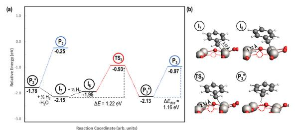
Fig. 7 Reaction energy diagram (a) with optimized intermediate structures (b) of benzyl alcohol hydrogenation to toluene (P\*) on reduced anatase TiO2 (001) with an Ovac. Structures with gas phase molecules are circled in blue, adsorbed species in black, and transition states in red. Only the uppermost atomic layer is shown for the sake of clarity. Ti (gray), O (red), C (black), H (white), and O<sub>vac</sub> (dashed circle) are depicted.
