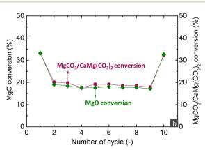
Fig. 4 (a) Outlet CO<sub>2</sub> concentration during the decarbonation stage of different cycles and (b) MgO and MgCO<sub>3</sub>/CaMg(CO<sub>3</sub>)<sub>2</sub> conversions over cycles for the  $MgCa_{0.05}A_{0.20}$  material when investigated via carbonate looping experiments in a fixed bed reactor (carbonation stage: 30%  $CO_2/He$ , 300 °C, 300  $h^{-1}$ ; decarbonation stage: 450 °C, 100% He, 720  $h^{-1}$ ).
