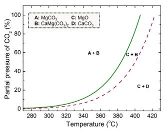
Fig. 1 Equilibrium curves of the carbonation of pure MgO (solid line) and MgO-CaCO3 (dashed line) with a CaCO3 to MgO molar ratio of 0.05 at 1 bar (recreated from ref. 16). In the figure, A refers to MgCO<sub>3</sub>, B to  $CaMg(CO_3)_2$ , C to MgO and D to  $CaCO_3$ .
