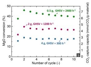
Fig. 5 (a) CO<sub>2</sub> capture efficiency during the carbonation stage of the 1st and 10th cycles and (b) CO<sub>2</sub> capture capacity and MgO conversion over cycles for the  $MgCa_{0.05}A_{0.20}$  material when investigated via carbonate looping experiments in a fixed bed reactor with different space velocities for the carbonation stage (carbonation stage: 30% CO<sub>2</sub>/He, 300 °C; decarbonation stage: 450 °C, 100% He, 720 h<sup>-1</sup>).
