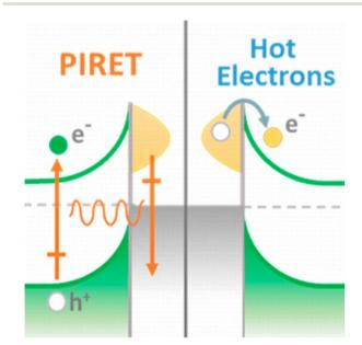
Fig. 5 Schema of the electronic conductions by plasmonic metals *via* charge carrier excitation in semiconductors through plasmoninduced resonance energy transfer (PIRET) and hot electron injection processes. Reprinted with permission from ref. 176 (N. Wu *et al.*). Copyright 2015 J. Phys. Chem. C, ACS.
