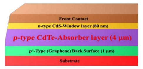
Fig. 7 Device structure of the graphene back surface-based CdTe solar cell. Reprinted with permission from ref. 207 (B. Pant et al.). Copyright 2021 Molecules, MDPI.
