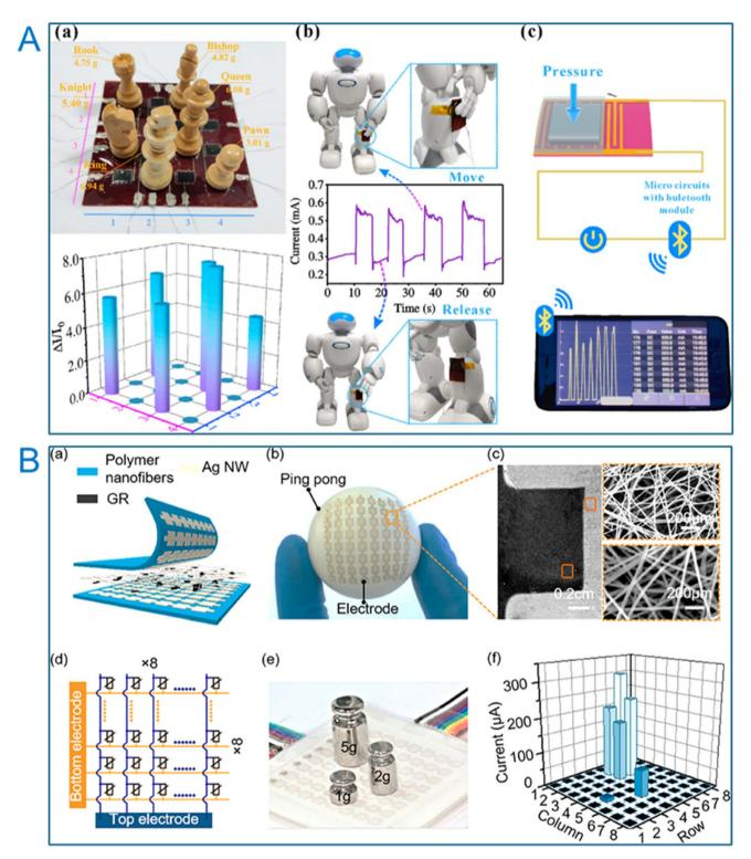
Fig. 3 (A) Flexible pressure sensor for array pressure distribution and human-robot interaction.<sup>27</sup> (B) Fiber electronics for pressure detection and learning in table tennis.28
