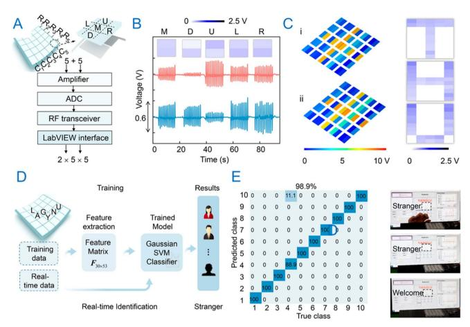
Fig. 4 Single-pixel sensing for machine learning-assisted individual identification. (A) Signal acquisition and processing system diagram. (B) Single-pixel tactile voltage signal during contact. (C) Theoretical simulation of voltage signal distribution. (D) Training and real-time identification process. (E) Classification of 10 individuals and video snapshots of real-time personal identification.<sup>34</sup>
