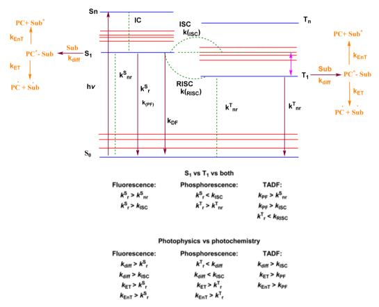
Fig. 45 Jablonski diagram and potential photochemical pathways for excited states of luminescent compounds such as TADF materials. Reproduced from ref. 208, https://doi.org/10.1039/D1CS00198A, under the terms of the CC BY-NC 3.0 license, https://creativecommons.org/licenses/by-nc/3.0/.
