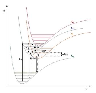
Fig. 44 Jablonski-type graph along Morse potentials illustrating the photophysical mechanism in TADF molecules. Reproduced from ref. 208, https://doi.org/10.1039/D1CS00198A, under the terms of the CCBY-NC 3.0 license, https://creativecommons.org/licenses/by-nc/3.0/.
