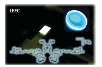
Fig. 110 The chemical structure of the TADF compound superimposed on a photograph of its LEEC. Reproduced from ref. 330, https://doi.org/10.1021/acs.chemmater.5b03245, under the terms of the CC BY 4.0 license, https://creativecommons.org/licenses/by/4.0/
