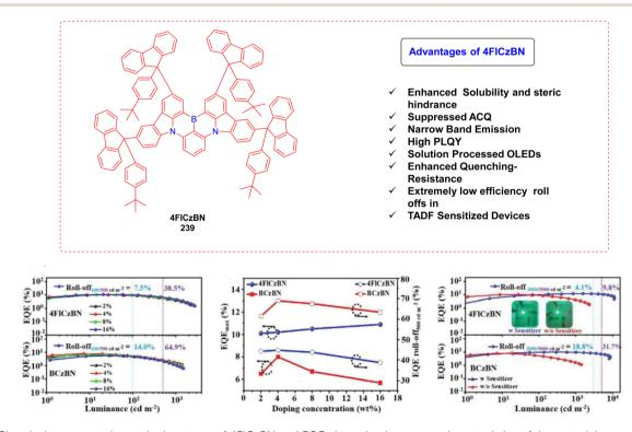
Fig. 88 Chemical representation and advantages of 4FICzBN and EQE electroluminescence characteristics of the material.
