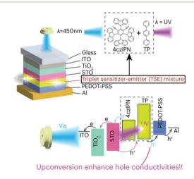
Fig. 98 Visible light-assisted charge extraction in high bandgap  $SrTiO_3$  through the integration of triplet sensitizer-emitter thin film. Reproduced from ref. 302 with permission from American Chemical Society, Copyright © 2024.
