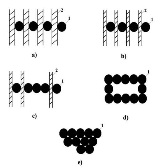
Fig. 7 Schematic representation of options for the formation of electronic and tunnel conductivity in nanocomposites based on polyolefin CB: (a) nanoparticles (1) separated by a thick dielectric layer (2); (b) nanoparticles (1) separated by a thin layer of dielectric (2); (c) mixed – electron (1) and tunnel (2) conductivity; (d) chain clusters; (e) nanoparticle agglomerates (1).<sup>143</sup>
