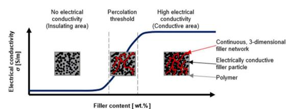
Fig. 5 The mechanism of electrical conductivity in polymer nanocomposites depending on the amount of introduced filler.<sup>152</sup>
