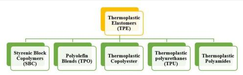
Fig. 3 Types of thermoplastics elastomers.<sup>70</sup>
