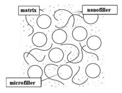
Fig. 1 Morphology of micro- and nanofilled composites.<sup>32</sup>
