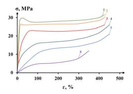
Fig. 11 Effect of the content of the elastomer component on the stress-strain curves of polymer blends based on compatibilized HDPE + SCS-30, wt%: (1) - initial HDPE; (2) - 10; (3) - 20; (4) - 30; (5) - 40; (6) - 50.183
