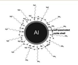
Fig. 4 Schematic representation of surface-modified aluminum nanoparticles.104
