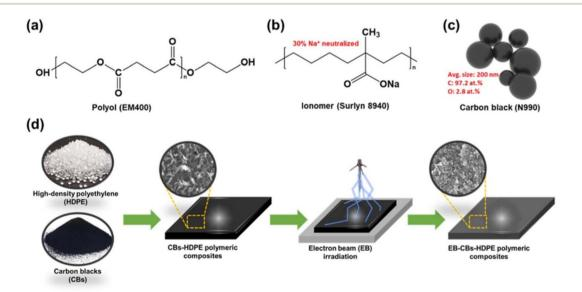
Fig. 8 Schematic illustration of the process of manufacturing electron-irradiated CB + HDPE nanocomposites. Chemical structures of (a) polyol (EM400), (b) ionomer (Surlyn 8940), and (c) CB (N990). (d) HDPE. 144
