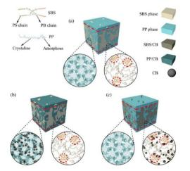
Fig. 9 Schematic representation of the distribution of CB in various forms: (a) without CB. (b) CB in PP. (c) CB in SBS. 156
