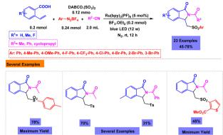
Scheme 25 Synthesis of sulfonated 1-isoindolinones *via* ruthenium-catalyzed one-pot four-component reaction of 2-vinylbenzoic acids, aryldiazonium tetrafluoroborates, the sulfur dioxide surrogate DABCO-(SO<sub>2</sub>)<sub>2</sub>, and nitriles.
