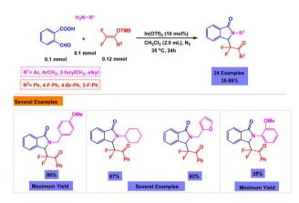
Scheme 27 Synthesis of 3-oxoisoindoline-1-difluoroalkyl derivatives via In(OTf)<sub>3</sub>-catalyzed one-pot, three-component Mannich/lactamization cascade reactions.
