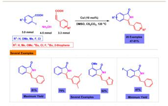
Scheme 1 Synthesis of isoindolin-1-ones via Cul-catalyzed one-pot three-component reaction of 2-iodobenzoic acids, alkynylcarboxylic acids and ammonium acetate.
