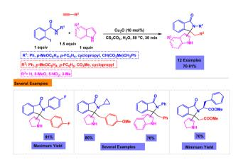
$\label{eq:Scheme} \begin{tabular}{lll} Scheme & 3 & Synthesis & of & 3-alkyl/aryl-3-(pyrrole/indole-2/3-yl)-2-phenyl-2,3-dihydro-isoindolinones & via & Cu_2O-catalyzed & multi-component one-pot reaction involving 2-iodo-N-phenylbenzamides, terminal alkyne and substituted indoles/pyrroles. \\ \end{tabular}$
