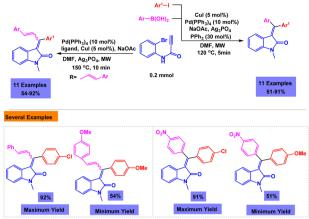
Scheme 24 Synthesis of 3-(1,3-diarylallylidene) oxindoles through palladium-catalyzed one-pot three-component reaction of N-aryl-propiolamides, aryl iodides and boronic acids.
