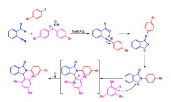
Scheme 7 Rational pathway for synthesis of 2,3-diarylisoindolin-1-one derivatives through copper-catalyzed one-pot, three-component annulations of 2-formylbenzonitriles, arenes, and diaryliodonium salts.
