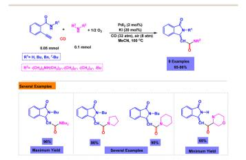
**Scheme 14** Synthesis of 3-[(dialkylcarbamoyl)methylene]isoindolin-1-ones through Pdl<sub>2</sub>-catalyzed oxidative carbonylation conditions.
