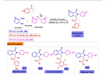
Scheme 10 Synthesis of dihydroisoindolo[2,1-a]quinolin-11(5H)-ones through  $Cu(OTf)_2$ -catalyzed one-pot three-component cascade cyclization among 2-formylbenzonitriles, alkyl aryl ketones/prop-1-en-2-ylbenzene and diaryliodonium salts.
