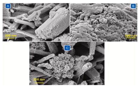
FESEM image of (A) FeCo<sub>2</sub>O<sub>4</sub> (B) PANI and (C) FeCo<sub>2</sub>O<sub>4</sub>/PANI. 132
