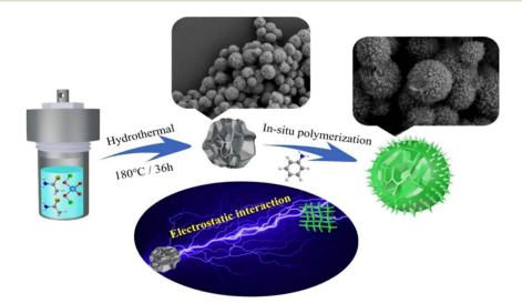
An illustration of the synthesis process of MoS<sub>2</sub>/PANI hybrids through in situ oxidative polymerization.<sup>141</sup>
