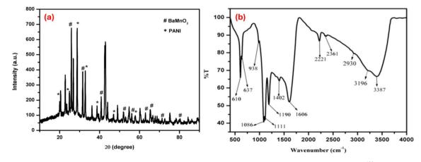
Fig. 4 (a) XRD patterns of PANI-BaMnO<sub>3</sub> nanocomposite and (b) FT-IR spectrum of PANI-BaMnO<sub>3</sub> nanocomposite.<sup>128</sup>
