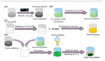
Fig. 7 Schematic showing the synthesis of rGO/TiO<sub>2</sub>/PANI nanocomposite via in situ emulsion polymerization: (a) preparation of rGO/ TiO<sub>2</sub> suspension, (b) addition of 3.2 mmol ANI monomer, (c) addition of 0.18 g APS and SDBS with stirring and (d) sonication drop-by-drop addition of APS solution with shaking for 3 hours. 139
