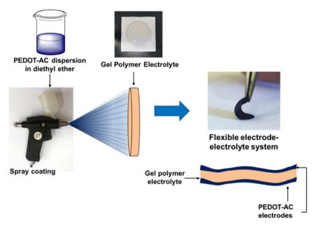
Fig. 19 Preparation of flexible electrode-electrolyte system. 174
