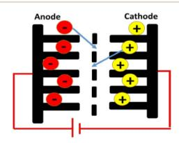
Fig. 1 Major components of a supercapacitor.74
