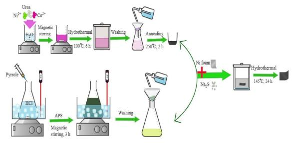
Fig. 14 Schematic representation of NiCo<sub>2</sub>S<sub>4</sub>@PPy nanomaterial fabrication. <sup>160</sup>
