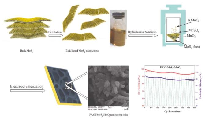
Fig. 11 Synthesis route for ternary PANI/MoS<sub>2</sub>-MnO<sub>2</sub> hybrid nanocomposite. 147
