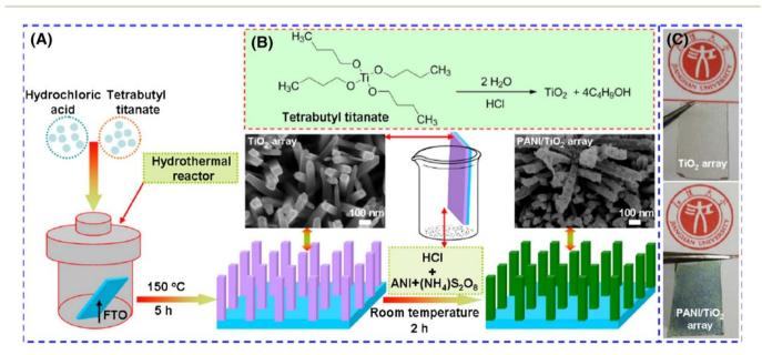
Fig. 6 (A) Synthesis of tetragonal prism array of  $TiO_2$  deposited on fluorine-doped tin oxide (FTO) and followed by PANI coating, (B) synthesis of  $TiO_2$  array *via* hydrolysis process, and (C) optical images of  $TiO_2$ /FTO and PANI/ $TiO_2$ /FTO.<sup>138</sup>
