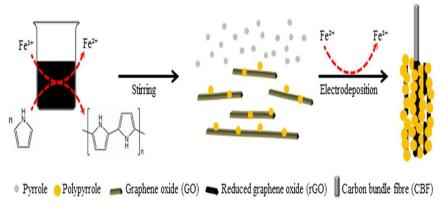
Fig. 15 Schematic diagram of the synthesis process of CBF/PPy-rGO-2.58
