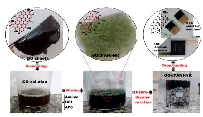
Fig. 10 Image showing the simple and ecofriendly synthesis and development procedures for rGO/PANI nanocomposites as active materials and supercapacitor electrodes.<sup>142</sup>
