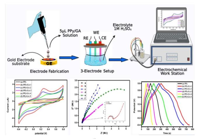
Fig. 16 Electrode fabrication towards electrochemical properties. 157
