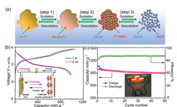
Fig. 4 (a) Schematic illustration for the mechanism of  $Se_4P_4$  during sodiation/desodiation, (b) charge/discharge curves (inset is the schematicillustration of  $Se_4P_4 - Na_3(VO_{0.5})_2(PO_4)_2F_2/C$  full cell), and (c) cycling performance of  $Se_4P_4 - Na_3(VO_{0.5})_2(PO_4)_2F_2/C$  full cell (inset is digital picture of afull cell that lights LEDs).<sup>72</sup>
