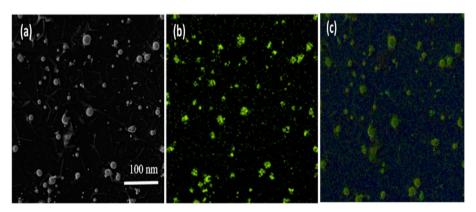
Fig. 7 SEM measurements of (a) SNPs with capsicum (b) SNPs with garlic (c) SNPs with ginger.<sup>236</sup>
