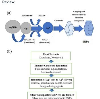
Fig. 5 (a) The supposed biosynthesis mechanism of SNPs.<sup>177</sup> (b) Flowsheet diagram showing mechanistic pathway of SNPs.
