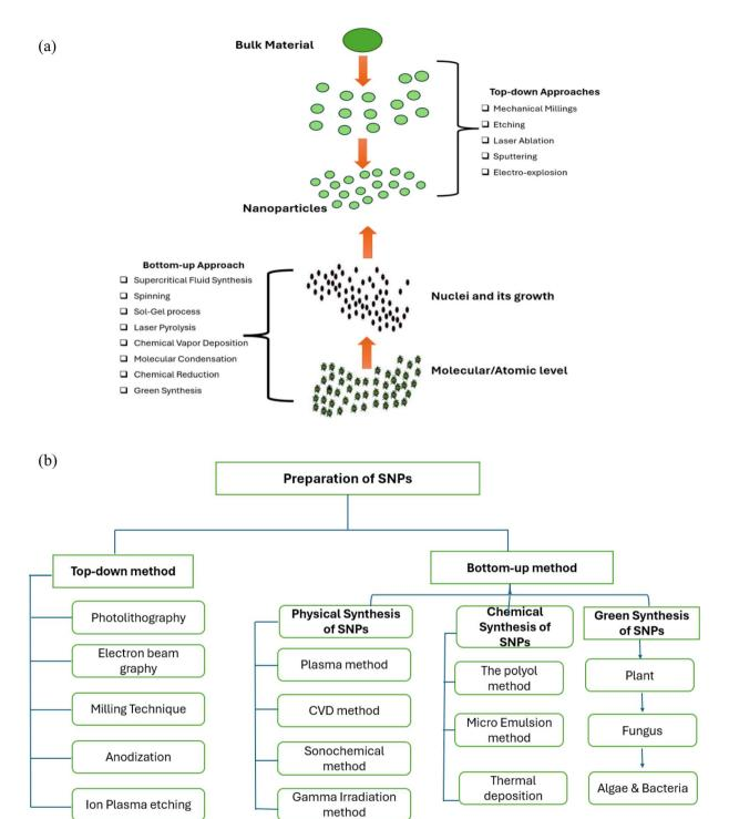
Fig. 1 (a) Methods for producing NPs.<sup>29</sup> (b) Enlisting the conventional and green synthesis methods of SNPs (reconstructed and modified from ref. 30).
