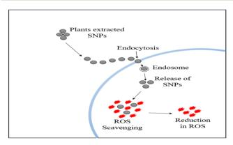
Fig. 17 Radical oxygen scavenging mechanism.<sup>266</sup>
