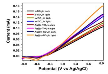
Fig. 11 Linear scan voltammograms of the p-TiO $_2$  and m-TiO $_2$  NPs as well as Ag@p-TiO $_2$  and Ag@m-TiO $_2$  nanocomposites photoelectrodes in the dark and under visible light irradiation. <sup>253</sup>
