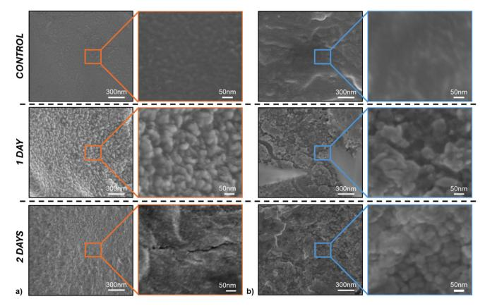
Fig. 7 SEM images of freeze-dried 3D-printed object prepared with (a)  $PCL_{11k}$ -BTPA and (b)  $PCL_{11k}$ -acrylate in the presence of IBoA, PEGDA and 10 wt% toluene, following selective etching of the PCL domains. Images show the control sample before etching (top), after 1 day of treatment (middle), and after 2 days of treatment (bottom) in a 0.5 M NaOH aqueous solution at 60 °C.
