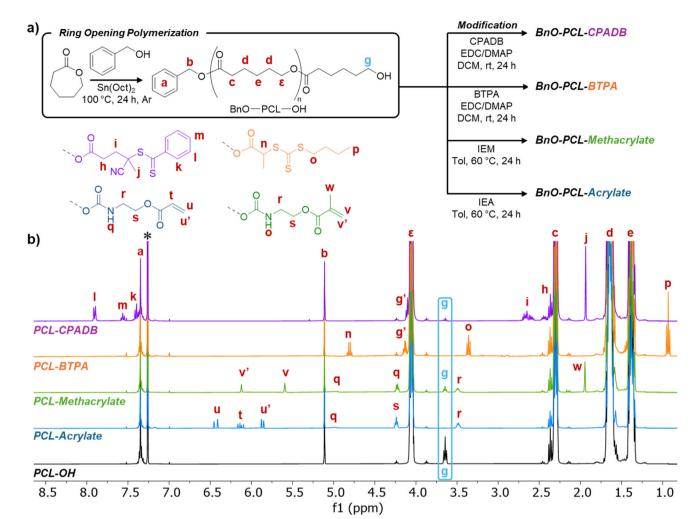
Fig. 2 Synthesis and characterization of functionalized PCL polymers. (a) Synthetic route for RAFT-terminated-PCLs (PCL-BTPA and PCL-CPADB) and acrylate/methacrylate-terminated-PCL (PCL-acrylate and PCL-methacrylate) via a two-step process. (b) <sup>1</sup>H NMR spectra of the starting PCL-OH and the four modified PCL polymers: PCL-acrylate, PCL-methacrylate, PCL-BTPA and PCL-CPADB (CDCl<sub>3</sub> (\*), 400 MHz, 298 K).
