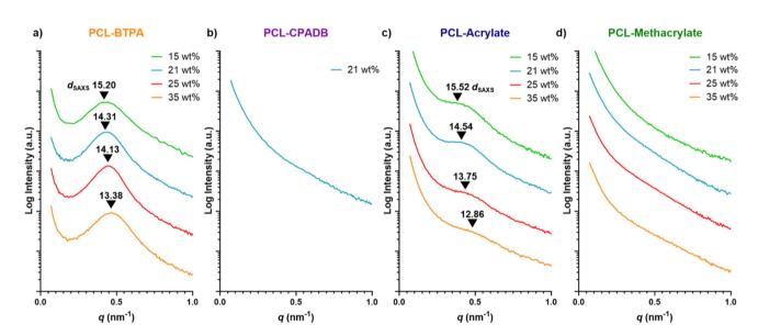
Fig. 4 SAXS profiles and the corresponding domain spacing ( $d_{SAXS}$ ) values for materials 3D printed with varying loadings of (a) PCL<sub>3k</sub>-BTPA, (b) PCL3k-CPADB, (c) PCL3k-acrylate, and (d) PCL3k-methacrylate. Loading: 15 wt% (green), 21 wt% (blue), 25 wt% (red) and 35 wt% (orange). [AA]/ [PEGDA] = 9/1 (molar ratio); TPO = 1 wt%.
