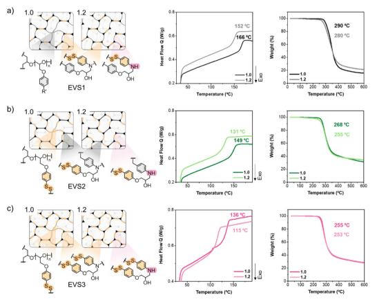
Fig. 3 Schematic representation of the 1.0 and 1.2 formulated networks and the corresponding DSC (with  $T_q$  insets) and TGA (with  $T_{d5\%}$  insets) traces. (a) EVS1, (b) EVS2 and (c) EVS3.
