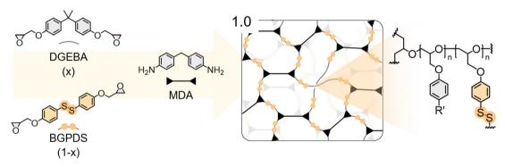
Fig. 9 Formulation of VES with varying contents of DGEBA and the schematic representation of the resulting stoichiometric network.
