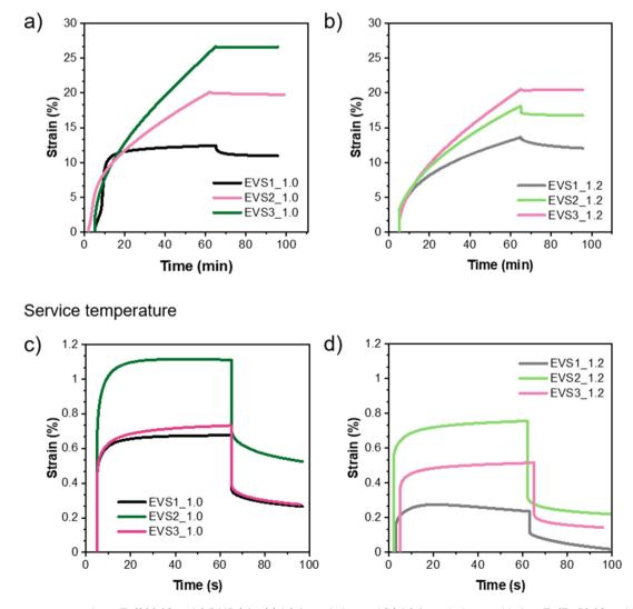
Fig. 6 Creep recovery test above  $T_g$  (200 °C and 0.5 MPa) for (a) 1.0 formulation and (b) 1.2 formulations and below  $T_g$  ( $T_g$ -50 °C and 5 MPa) for (c) 1.0 formulation and (d) 1.2 formulations.
