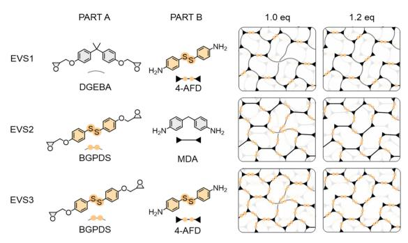
Fig. 2 Studied three epoxy vitrimer systems (EVS). Formulations (left) and schematic representations of the corresponding stoichiometric and non-stoichiometric networks.
