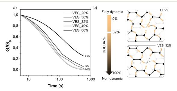
Fig. 11 (a) Normalized stress relaxation curve at 200 °C of the VES formulations. (b) Comparison of structural ESV systems and VES and their dynamicity correlation with DGEBA content.
