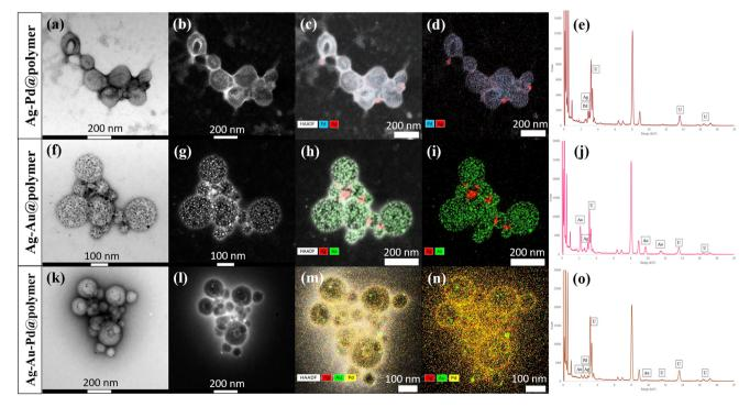
Fig. 3 STEM images of Ag-Pd, Ag-Au and Ag-Au-Pd@PEG113-b-PDMAEMA32-b-PHPMA398-CDTPA PMNCs in (a), (f) and (k) bright-field and (b), (g) and (l) HAADF modes. (c), (h) and (m) Overlapped bright-field and STEM-EDX mapping. (d), (i) and (n) STEM-EDX-mapping. (e), (j) and (o) EDX elemental analysis.
