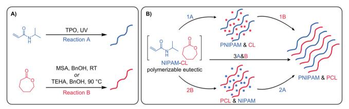
Scheme 1 (A) Schemes indicating reaction conditions used to prepare PNIPAM and PCL linear polymers. (B) Scheme showing sequential (reaction (1) & (2)) and simultaneous (reaction (3)) preparation of PNIPAM and PCL polymer blends from a PE mixture. Reactions labelled 'A' use photoinitiator and UV irradiation. Reactions labelled 'B' use an ROP catalyst & initiator.
