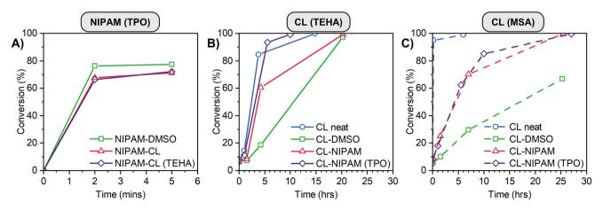
Fig. 3 Homopolymer control experiment conversion data for (A) NIPAM initiated by TPO, (B) CL catalysed by TEHA and (C) CL catalysed by MSA.
