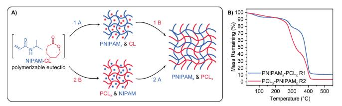
Fig. 6 (A) Scheme showing the sequential preparation of PNIPAM, & PCL, IPNs. Reactions A and B have the same conditions as in Scheme 1A with the addition of PEGDA for reaction (A), and bis(carbonate) for reaction (B). PCL-PNIPAMx semi-IPNs were prepared following reaction (2) without bis (carbonate) crosslinker present. (B) TGA thermograms of IPNs.
