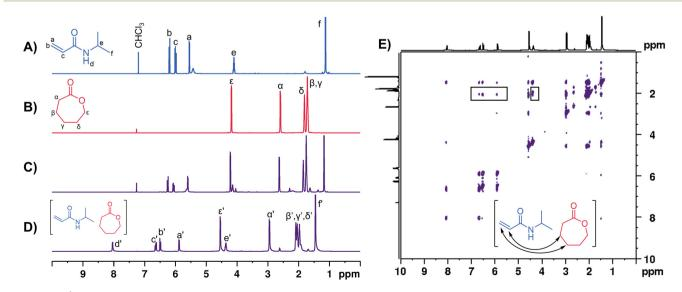
Fig. 2 (A-D)  $^{1}$ H NMR spectra of (A) NIPAM, (B) CL, (C), NIPAM-CL<sub>0.67</sub> dissolved in CDCl<sub>3</sub>, (D) neat NIPAM-CL<sub>0.67</sub> PE containing a capillary filled with CDCl<sub>3</sub>. (E)  $^{1}$ H- $^{1}$ H ROESY NMR spectrum of NIPAM-CL<sub>0.67</sub> with discernible correlations identified.
