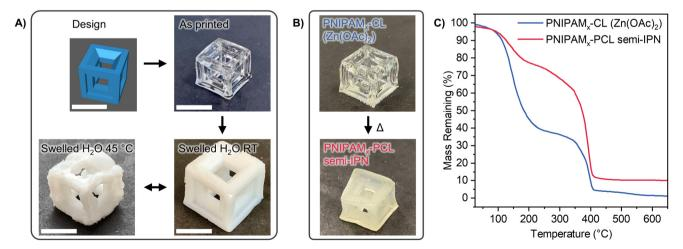
Fig. 7 (A) Images of PNIPAM $_x$ -CL 3D printed cube structure showing reversible thermoresponsive swelling in water. Scale bar in all figures represents 1 cm. (B) Images of PNIPAM $_x$ -CL (with zinc acetate present) and PNIPAM $_x$ -PCL semi-IPN 3D printed materials. (C) TGA thermograms of PNIPAM $_x$ -CL with zinc acetate present (blue) and PNIPAM $_x$ -PCL semi-IPN (red).
