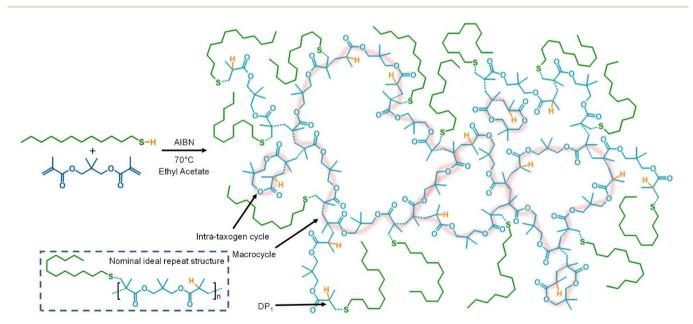
Fig. 4 TBRT synthesis of p(DDT-NPGDMA) via the homopolymerisation of neopentyl glycol dimethacrylate (NPGDMA) with 1-dodecanethiol (DDT). Macrocycles may be formed within the structure or intramolecular cyclisation of NPGDMA may lead to small cycles. Inset shows the nominal repeat unit under ideal conditions.
