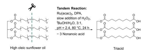
Scheme 1 Ruthenium catalyzed oxidative cleavage of high oleic sunflower oil (DPA: pyridine-2,6-dicarboxylic acid and Ru(acac)<sub>3</sub>: ruthenium(III) acetylacetonate).
