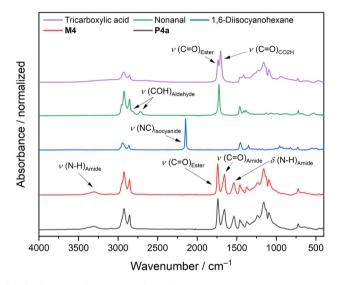
Fig. 2 Stacked IR spectra of sunflower oil-based tricarboxylic acid, nonanal (4), 1,6-diisocyanohexane (a), model compound M4, and polymer P4a. Each IR spectrum is normalized to the strongest absorbance vibration.
