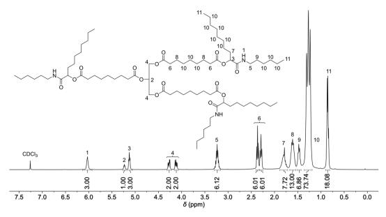
Fig. 1 <sup>1</sup>H NMR spectrum of M4 in CDCl<sub>3</sub>. Integrals are referenced to protons 4 of the glyceryl moiety.
