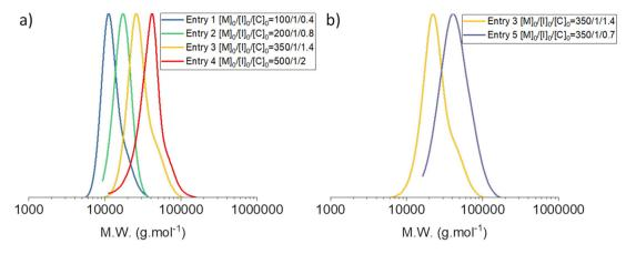
Fig. 9 Size-exclusion chromatograms of the PDMS prepared by the AROP of  $D_3$  and shown in Table 2.
