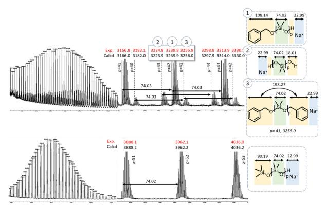
MALDI-TOF mass spectra of precipitated PDMS initiated by benzyl alcohol (top) and trimethyl silanol (bottom).
