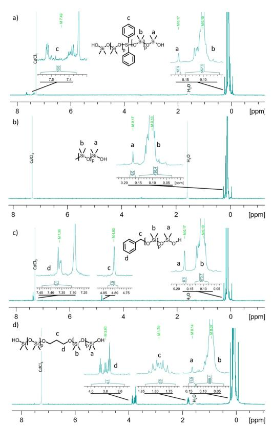
Fig. 2 <sup>1</sup>H NMR spectra in CDCl<sub>3</sub> of precipitated PDMS initiated by (a) diphenylsilanediol, (b) trimethylsilanol, (c) benzyl alcohol, and (d) propane diol.
