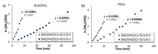
Fig. 6 First-order kinetics plot of the ROP initiated by (a) diphenylsilanediol and (b) propanediol.
