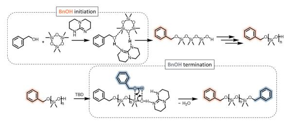
Scheme 4 Mechanism of BnOH initiated AROP of D<sub>3</sub> catalyzed by TBD.
