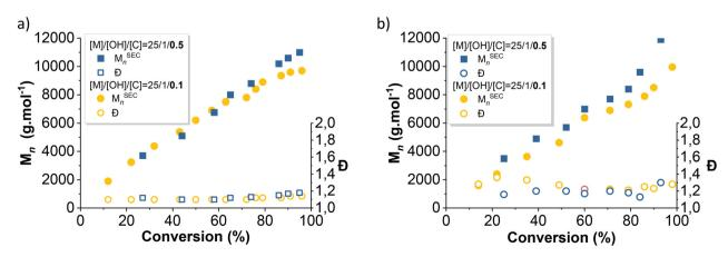
Fig. 7 Evolution of the number average molar mass and dispersity with  $D_3$  conversion of PDMS prepared by a TBD-catalyzed AROP of  $D_3$  initiated with (a)  $\Phi_2$ Si(OH)<sub>2</sub> and (b) Pdiol.
