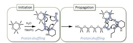
$\textbf{Scheme 1} \quad \text{``Proton shuffling'' mechanism of initiation and propagation of } D_3 \textit{via} \text{ TMnPG-catalyzed AROP.} \\ ^{16}$
