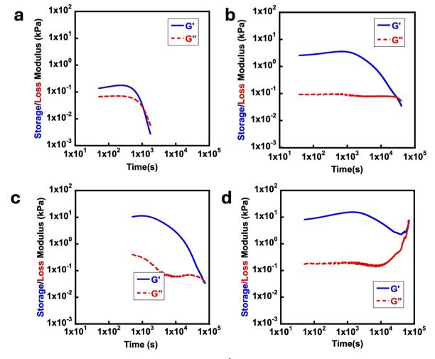
Fig. 3 Typical rheology time sweeps at 15 °C using a frequency of 10 rad s<sup>-1</sup> for deprotected poly(ONBM<sub>15</sub>-DMAm<sub>81</sub>) with (a) 0.5 M, (b) 1.0 M, (c) 1.5 M and, (d) 2.0 M concentrations of EDC
