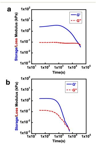
Fig. 4 Typical rheology time sweeps at 15 °C using a frequency of 10 rad  $s^{-1}$  with 1 M EDC for deprotected (a) poly(ONBM<sub>15</sub>-DMAm<sub>81</sub>) and (b) poly(ONBM<sub>15</sub>-DMAm<sub>122</sub>).
