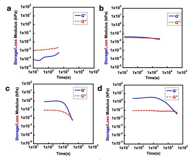
Fig. 2 Typical rheology time sweeps at 15 °C using a frequency of 10 rad s<sup>-1</sup> for poly(ONBM<sub>15</sub>-DMAm<sub>81</sub>) exposed to 360 nm UV for (a) 8 h then 1 M EDC, (b) 8 h then 2 M EDC (c) 16 h then 1 M EDC and (d) 24 h then 1 M EDC.
