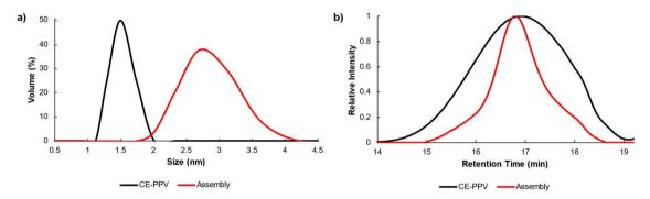
Fig. 3 (a) DLS in 1:1 CHCl<sub>3</sub>/CH<sub>3</sub>CN and (b) GPC characterization in THF, against linear PS standards, of homopolymer CE-PPV (13b) (black) and the supramolecular bottlebrush CE-PPV-PS-DBA+ (red).
