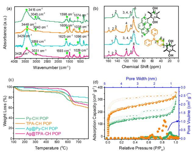
Fig. 1 (a) FTIR, (b) sold state NMR (c) TGA profiles of Py-CH, TPA-CH, Ag@Py-CH, and Ag@TPA-CH POPs, and (d) BET and pore sizes profile of Py-CH, and TPA-CH POPs.
