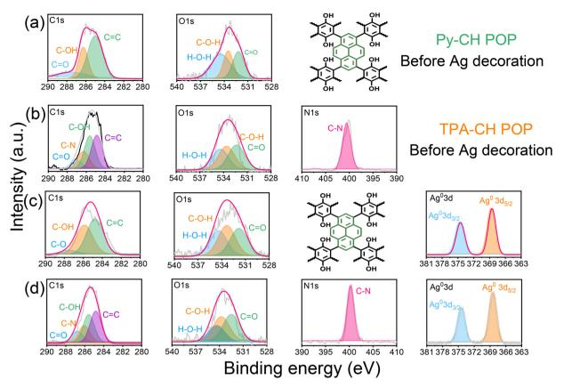
Fig. 2 XPS spectrum profiles of Py-CH (row a), TPA-CH (row b) POPs, 3Ag@Py-CH (row c), and 3Ag@TPA-CH POPs (row d).
