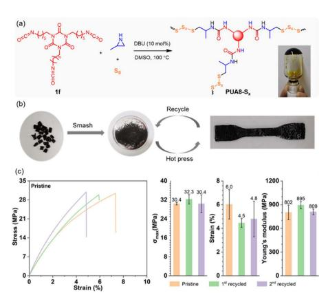
Fig. 4 (a) Synthesis of polyurea vitrimer  $PUA8-S_x$ . (b) The recycling process for the polyurea vitrimer sheet. (c) Stress-strain curves, maximum stress, breaking strain, and Young's modulus of vitrimer  $PUA8-S_x$  before recycling and after two recycling cycles.
