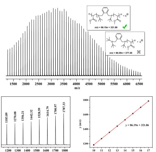
Fig. 3 MALDI-TOF MS spectrum of low-MW PMAs and plots of m/z values (y) vs. the number of MS repeat units (n) for molecular ion peaks.
