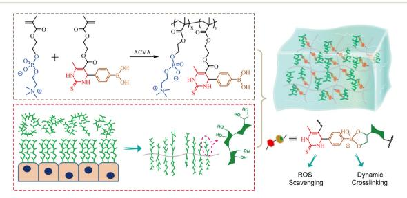
Fig. 1 Schematic illustration of the molecular structure of functional zwitterionic PMPD copolymer and the preparation of mucus-inspired hydrogel through dynamic phenylboronic ester cross-linking.
