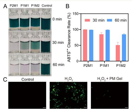
Fig. 5 (A) Photographs of ABTS<sup>-+</sup> solutions co-incubated with P2M1, P1M1, and P1M2 hydrogels for (i) 0 min, (ii) 30 min, and (iii) 60 min. (B) The ABTS<sup>++</sup> scavenging efficiency of PM hydrogels after co-incubation for 30 and 60 min. (C) Intracellular ROS-scavenging capability of PM hydrogel as monitored by DCFH-DA probe. Scale bar = 100  $\mu$ m.
