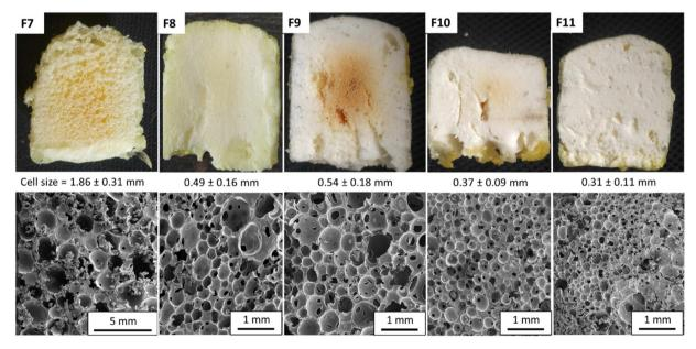
Fig. 7 Images and SEM of the different foams obtained from r.t. formulations under catalyst free conditions. Conditions: TMPTC, epoxide, amine, thiol with [5CC] : [epoxide] :  $[NH_{2 \text{ total}}]$  : [SH] = 1 : 1 : 1.5 : 0.5, foaming RT.
