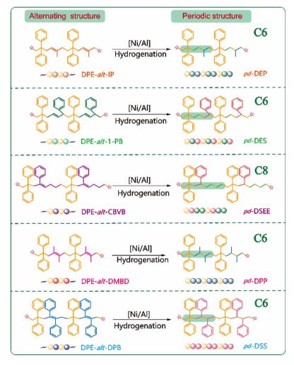
Scheme 2 Periodic polymers prepared by the hydrogenation of alternating polymers.
