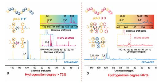
Fig. 3 IG-<sup>13</sup>C NMR spectra of alternating polymers and periodic polymers: (a) for the copolymer of DPE with DMBD and (b) for the copolymer of DPE with DPB.
