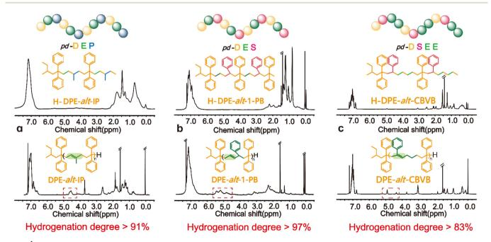
Fig. 2 <sup>1</sup>H NMR spectra of alternating polymers and periodic polymers: (a) for the copolymer of DPE with IP; (b) for the copolymer of DPE with 1-PB; and (c) for the copolymer of DPE with CBVB.
