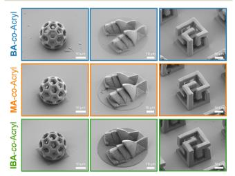
Fig. 4 SEM images of 3D structures printed with high resolution and fine features printed using all three inks at the same printing parameters (32.5 mW and 15 mm s<sup>-1</sup>).
