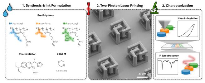
Scheme 1 Overall approach used to determine the structure-property relationships between three polymer inks BA-co-Acryl, MA-co-Acryl, and IBA-co-Acryl through 1) rational design of copolymer materials for ink formulation, 2) determination of optimum parameters using 2PLP and 3D printing microstructures, and 3) characterization through infrared spectroscopy and nanoindentation to determine chemical and mechanical properties, respectively.
