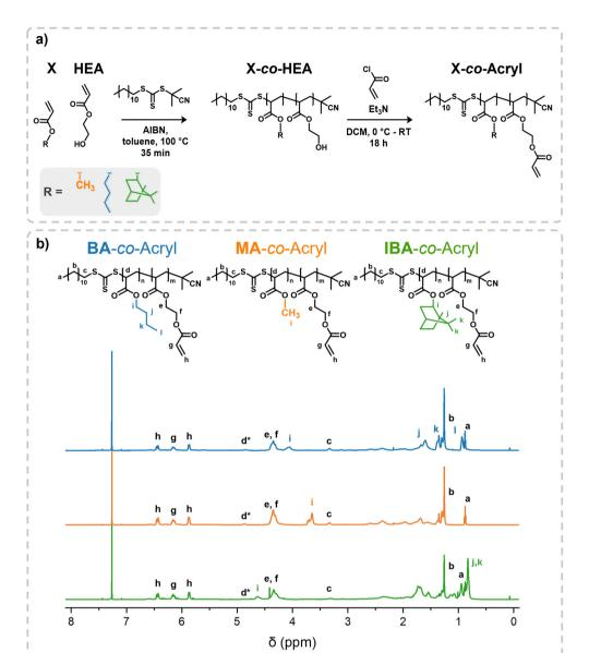
Fig. 1 a) Synthetic pathway for the preparation of each macromolecules using RAFT-controlled radical polymerization followed by functionalization with crosslinkable acrylate groups and b) 1H-NMR spectra (CDCl<sub>3</sub>, 600 MHz, 128 s, 295 K) of BA-co-Acryl (top, blue), MA-co-Acryl (middle, orange) and IBA-co-Acryl (bottom, green) polymers after post functionalization, where d\* represents the protons of the monomer directly adjacent to the S of the chain transfer agent.
