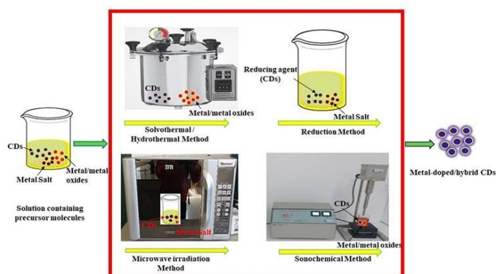
Figure 6. Schematic representation of various methods used for synthesizing the metal-doped and hybrid CDs. Reproduced with permission. 80 Copyright 2025, Elsevier.
