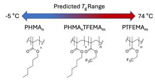
Fig. 2 Chemical structures of the homopolymers, PHMA and PTFEMA, and the resultant copolymer poly(n-hexyl methacrylate-co-2,2,2trifluoroethyl methacrylate) (PHMA<sub>n</sub>TFEMA<sub>m</sub>). The monomer ratios, n and m, were varied to access a range of glass transition temperatures,  $T_{a}$ .
