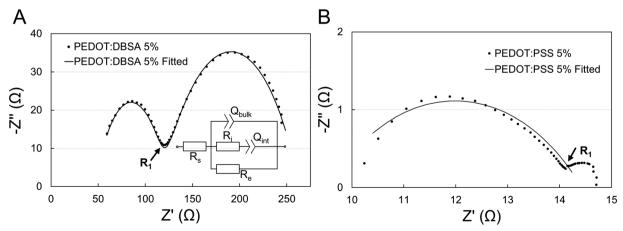
Fig. 5 Complex impedance plots of (A) – the PEDOT:DBSA and (B) – the PEDOT:PSS hydrogel measured and fitted with the inserted equivalent circuit at zero DC bias.  $R_s$  stands for serial contact resistance;  $R_i$  stands for ionic resistance; and  $R_e$  for electronic resistance. The total resistance of the hydrogels was determined as  $R_1 = R_i R_e / (R_e + R_i)$ .
