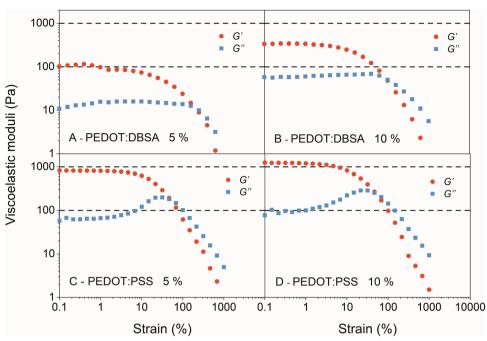
Fig. 3 Strain sweep test of the PEDOT:DBSA and the PEDOT:PSS doped with (A) and (C), 5 v/v% of DBSA; (B) and (D), 10 v/v% of DBSA. G' and G'' show the values of the measured storage and loss modulus, respectively. For better clarity, the dashed line marks the value of viscoelastic moduli of 100 and 1000 Pa.
