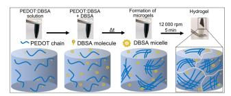
**Fig. 1** Proposed formation of the PEDOT:DBSA hydrogel. The addition of DBSA promotes hydrophobic interactions between the PEDOT chains, resulting in the formation of microgels, which are not connected in the whole sample volume.
