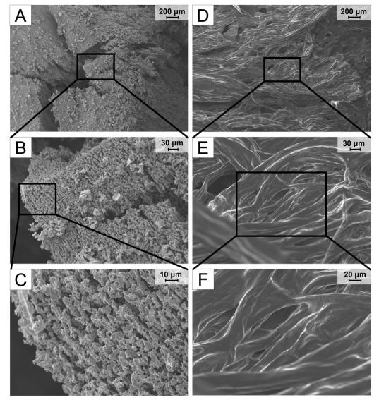
Fig. 4 Cross-section of lyophilized xerogels of PEDOT:DBSA (A)–(C) and of PEDOT:PSS (D)–(F), both doped with 5 v/v% of DBSA. Both samples are shown in three magnifications, so that the wider surroundings ( $100\times$ ; (A) and (D)) can be seen, as well as the details of the structure ((C)  $2000\times$ ; (F)  $1000\times$ ).
