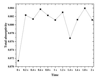
Fig. 3 The total absorptivity of the fluidized bed at different times with the gas flow set at 10 sccm and particle absorptivity 0.95; note that at time 0 s, the bed is in the fixed (non-fluidized) state.
