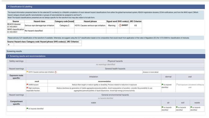
Fig. 3 Classification and labelling (top) and screening results and recommendations (bottom) of the SWCNT obtained by the platform.
