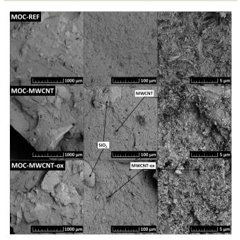
Fig. 5 SEM micrographs of the prepared MOC-based composites.
