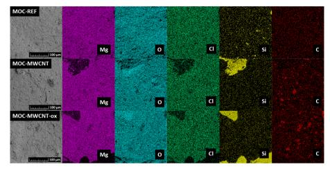
Fig. 6 EDS elemental maps of the prepared MOC-based composites.
