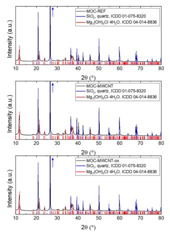
Fig. 4 Diffraction patterns of the samples MOC-REF (top), MOC-MWCNT (middle), and MOC-MWCNT-ox (bottom) obtained from XRD.
