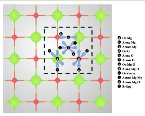
Fig. 1 Adsorption site and orientation map for considered starting configurations for CO2 adsorption on the clean bulk-cleaved MgO (100) surface (top-down view). Mg and oxygen atoms are represented in green and red, respectively.
