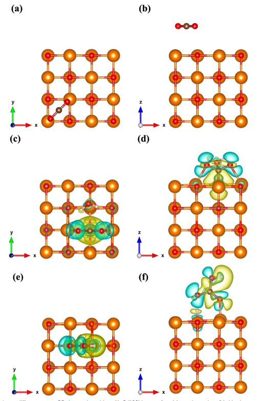
Fig. 10 Visualized charge difference upon  $CO_2$  interacting with an MgO (100) bare surface (a) top-down view, (b) side view, methanol/IPA-treated surface with carbonate-like species formation (c) top-down view, (d) side view, methanol/IPA-treated surface with bicarbonate-like species formation (e) top-down view, (f) side view.
