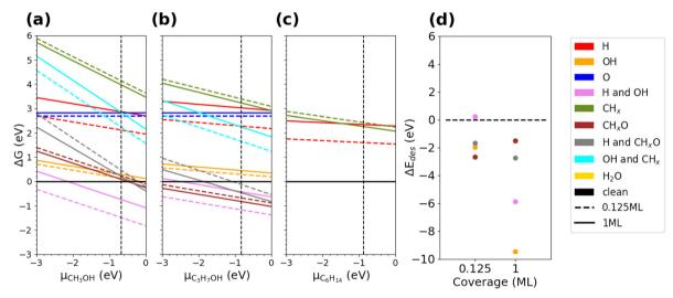
Fig. 8 Stability phase diagrams for an MgO (100) surface exposed to different solvents (a) methanol, (b) isopropanol, and (c) hexane, resulting in adsorption of different solvent-derived species as indicated by the legend. (d) Desorption energetics of the methanol/IPA-treated MgO (100) surface in equilibrium with vacuum.
