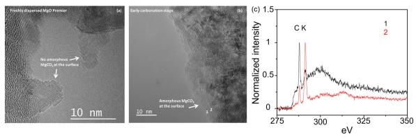
Fig. 6 Carbonation of MgO upon being exposed to exhaled air. (a) Freshly dispersed MgO Calix with clean surface. (b) Freshly dispersed sample A (MgO Calix) upon being exposed to human exhaled air. (c) EELS C-edge for region t 1 (fully carbonated) and region 2 (front of carbonation) in panel
