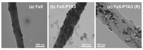
Fig. 2 TEM images of (a) Fe5, (b) Fe5-PTA3, and (c) Fe5-PTA3(R) prepared with Fe oxide from vendor B.
