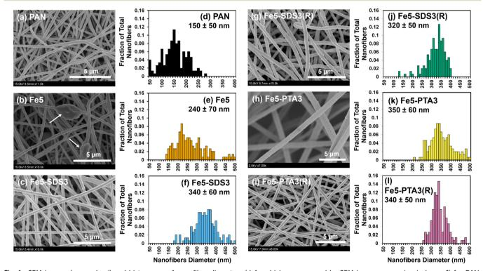
Fig. 1 SEM images (a-c and q-i) and histograms of nanofiber diameters (d-f and j-l; as measured by SEM image processing in ImageJ) for PAN, Fe5, Fe5-SDS3, Fe5-SDS3(R), Fe5-PTA3, and Fe5-PTA3(R). The Fe oxide particles obtained from vendor B were used for all of these materials. Average nanofiber diameters and standard deviation were determined by measuring at least n = 150 nanofibers for each material.
