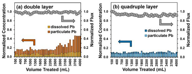
Fig. 7 Total Pb removal (left y-axis) and flux (right y-axis) during a single pass-through a (a) double (~240 μm) and (b) quadruple (~480 μm) layer filter of Fe5(B)-PTA3. Also shown are the relative contributions of dissolved and particulate Pb measured in the filter permeate. Experimental conditions: total feed volume = 4 L, flow rate = 20 mL min<sup>-1</sup>, influent conditions are described in Table S1,† effective nanofiber area = 12.6 cm<sup>2</sup>, and pH 8.5.
