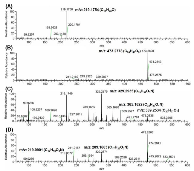
Fig. 6 HRMS spectra of (A and B) PS MPs zoomed in at retention times of 16.64 and 17.27, respectively. (C and D) TiAP\_With H<sub>2</sub>O<sub>2</sub> zoomed in at retention time of 16.72 and 17.33, respectively. Spectra were taken at a fragmentation intensity of 70 V.
