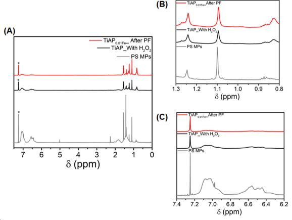
Fig. 5 (A) <sup>1</sup>H NMR spectra of PS MPs, TiAP\_With H<sub>2</sub>O<sub>2</sub>, and TiAP<sub>0.01Fe</sub>\_After PF. (B) and (C) The zoomed-in spectra between 0.8–1.3 ppm and 6.2– 7.5 ppm, respectively. Solvent peaks are marked with an asterisk (\*).
