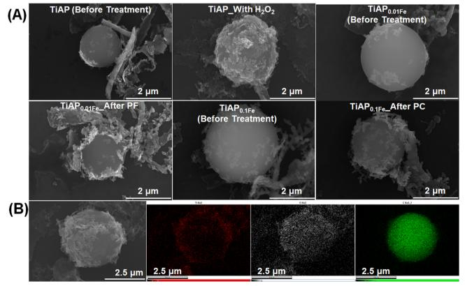
Fig. 3 (A) Representative HRSEM images before treatment and samples with a higher change in CI value after the photo-induced treatment process and (B) EDX mapping of the representative sample (TiAP\_Before Treatment), showing the distribution of C (PS MPs) colored in green, Ti in red, and O in white
