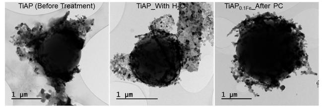
Fig. 4 Representative HR-TEM images of TiAP before treatment and samples with higher changes in the CI value (TiAP\_With H<sub>2</sub>O<sub>2</sub> and TiAP<sub>0.1Fe</sub>\_After PC).
