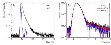
Fig. 5 (A) Fluorescence decay kinetics of aqueous dispersions of GO excited at 405 nm and recorded at 680 nm. (B) Fluorescence decay kinetics of aqueous dispersions of CeO<sub>2</sub> and CeGO20 excited at 340 nm and recorded at 370 nm.
