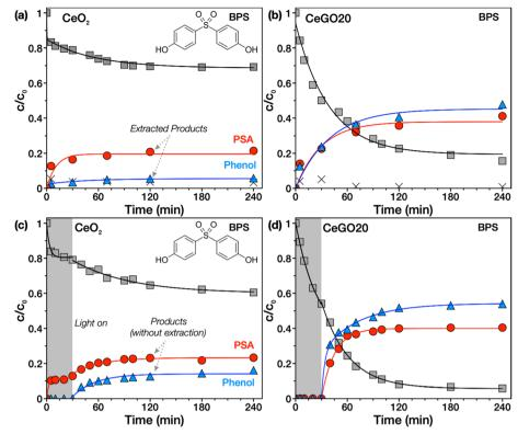
Fig. 6 Reactive adsorption of BPS on (a)  $CeO_2$  and (b)  $CeO_2$  nanoparticles grown on GO (representative sample CeGO20); solar-light enhanced photodecomposition of BPS on (c)  $CeO_2$  and (d) sample CeGO20. Color coding: black squares – BPS concentration in solution, black crosses – BPS extracted from the surface of the catalyst, red circles – PSA and blue triangles – phenol (both extracted in the case of dark tests or released and analyzed directly in solution in photocatalytic tests).
