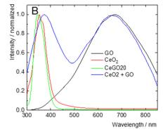
Fig. 4 (A) Normalized absorption spectra of water dispersions of GO, CeO2, and CeGO20. (B) Normalized luminescence spectra of water dispersions of GO, CeO<sub>2</sub>, CeGO20, and the physical mixture of CeO<sub>2</sub> and GO, excitation at 250 nm.
