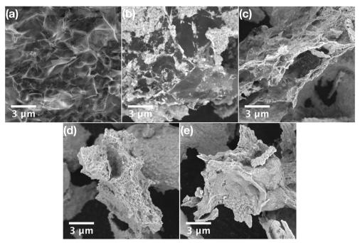
Fig. 2 SEM-CBS images of (a) GO, (b) CeGO20, (c) CeGO10, (d) CeGO05, and (e) pure CeO<sub>2</sub>.
