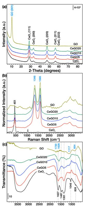
Fig. 1 (a) XRD patterns, (b) Raman spectra and (c) FTIR spectra of  ${\rm CeO_2}$ , GO and their composites.
