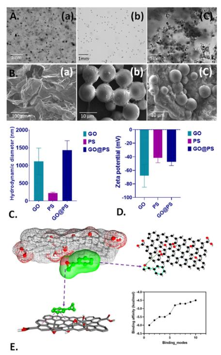
Fig. 2 Physicochemical characterization of the GO, PS, and GP@PS. (A) Optical microscopy images of (a) graphene oxide (GO), (b) polystyrene (PS), (c) GO@PS. (B) Scanning electron microscopy images of (a) GO, (b) PS, and (c) GO@PS. (C) Hydrodynamic diameters of GO, PS, and GO@PS determined by dynamic light scattering. (D) Zeta potentials of GO, PS, and GO@PS determined by dynamic light scattering. (E) Molecular interactions of GO and PS in GO@PS as determined by computational molecular docking.
