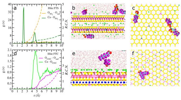
Fig. 6 Radial distribution functions (solid lines) and corresponding running coordination numbers (RCNs-dashed lines) between (a) 6:2 FTS and (d) 6:2 FTC with the basal surface adsorbed Ca<sup>2+</sup> ions and 'O' atoms of illite. Pictorial representations of (b and c) surface adsorbed 6:2 FTS and (e and f) 6:2 FTC and their clusters at the basal surface of illite.
