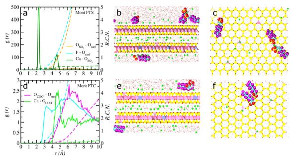
Fig. 5 Radial distribution functions (solid lines) and corresponding running coordination numbers (RCNs-dashed lines) between (a) 6:2 FTS and (d) 6:2 FTC with the basal surface adsorbed Ca<sup>2+</sup> ions and 'O' atoms of montmorillonite. Pictorial representations of (b and c) surface adsorbed 6:2 FTS and (e and f) 6:2 FTC and their clusters at the basal surface of montmorillonite.
