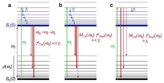
Fig. 29 Simplified Jablonski diagrams depicting the fluorescence processes in the three possible situations: (a) Standard fluorescence; (b) SEF in which the vibrational decay rate is faster than the SEF rate; and (c) SEF in which the vibrational decay rate is slower than the SEF rate. Reprinted with permission from ref. 303 Copyright 2007 American Chemical Society
