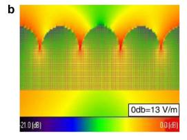
Fig. 43 (a) FDTD simulated electric-field distribution for a cauliflower-like Rh nanoparticle and (b) a flat Rh surface decorated with small nanohemispheres. The laser beam illuminates along the y-direction with x polarization. The scale bar is given at the bottom of (b). Figures are adapted from ref. 405 and 407 with permission. Copyright 2006 Springer Nature. Copyright 2006 Royal Society of Chemistry
