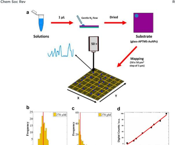
Fig. 58 The digital analysis in SERS measurement. (a) Schematics of the experimental procedure. (b) Histogram showing the frequency of normalized scores from "factor 1", which corresponds to the spectral signature of the analyte. The data is obtained from high concentration regime and (c) ultralow concentration regime. (d) Digital calibration curve at ultralow concentration. Figures are adapted from ref. 578 with permission. Copyright 2018 American Chemical Society.
