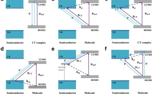
Fig. 44 Various mechanisms of a photo-induced CT process (blue line) and coupling scheme (purple line) in semiconductor-molecule systems. (a) Resonant excitation of the CT complex, (b) molecular HOMO-to-CB, (c) CT complex-to-CB, (d) VB-to-molecular LUMO, (e) surface state to molecular LUMO, and (f) molecular excited state-to-CB transitions. Figures are adapted from ref. 417 with permission. Copyright 2018 World Scientific Publishing Europe Ltd
