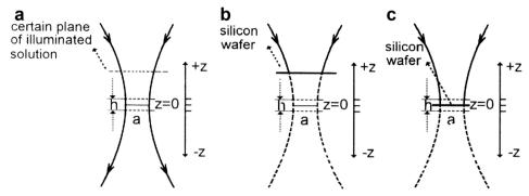
Fig. 48 (a) Illustration of the contribution to I<sub>Raman</sub> from a certain plane of illuminated solution. (b) and (c) Illustration of vertical movement of a flat Si waver for obtaining the confocal depth dependence of the Raman signal. Reproduced from ref. 402 with permission. Copyright 1998 Elsevier.
