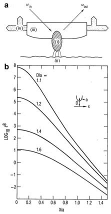
Fig. 11 (a) The optical probe particle (i) intercepts an incident laser beam, of frequency  $\omega_{\rm in}$ , and concentrates the field in a region adjacent to the sample surface (ii). The Raman signal from the sample surface is reradiated into the scattered field at frequency  $\omega_{
