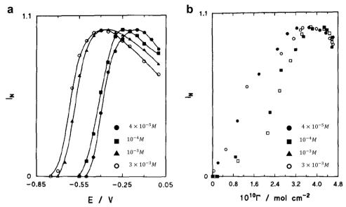
Fig. 50 (a) Plots of the intensity of the 1010 cm<sup>-1</sup> band on the electrode potential (E vs. SCE) for the varied bulk pyridine concentrations. (b) Data from panel a plotted versus surface concentration of pyridine  $\Gamma$ . Figures are adapted from ref. 119 with permission. Copyright 1991 Elsevier.
