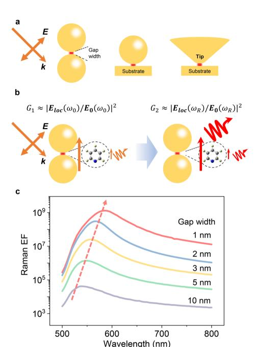
Fig. 23 (a) Representative nanostructures for gap-mode SERS/TERS, including nanoparticle dimer, nanoparticle on substrate and tip on substrate (b) The two-step process of enhancement of the electromagnetic field in SERS for nanoparticle dimer. (c) The spectra of the maximum Raman EFs for nanoparticle dimers with different gap widths.
