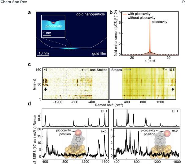
Fig. 38 (a) The schematics of picocavity formed by adatoms on Au nanoparticles. (b) Near field enhancement in the cavity. (c) Time-series anti-Stokes and Stokes SERS in the picocavity. (d) Comparison of two experimental spectra (bottom) with DFT simulated spectra (top) under the assumption of atomic-scale field confinement (inset shows geometries, red sphere shows field ocalization for simulations). Figures are reproduced from ref. 358 with permission. Copyright 2016 AAAS
