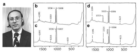
Fig. 4 (a) Photograph of Richard P. Van Duyne. Reproduced from ref. 58 with permission. Copyright 2020 Wiley. (b)–(e) Raman spectra of pyridine adsorbed on a Ag electrode. The solution contained 50 mM pyridine and 0.1 M KCI. Electrode potentials are -0.2 V, -0.4 V, -0.6 V and -0.8 V for (b)–(e). The Raman spectra were enhanced by image processing methods as the original spectra were blurry. Reproduced from ref. 2 with permission. Copyright 1977 Elsevier B.V.
