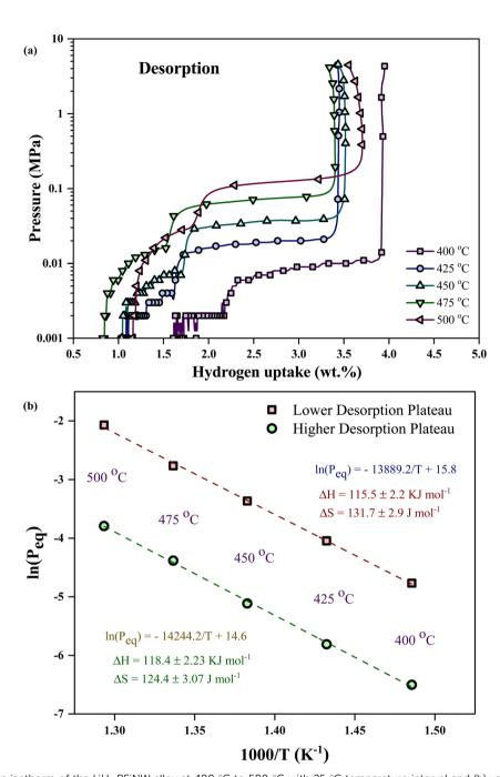
Fig. 3 (a) PCI desorption isotherm of the LiH-PSiNW alloy at 400  $^{\circ}$ C to 500  $^{\circ}$ C with 25  $^{\circ}$ C temperature interval and (b) van't Hoff plot for hydrogen desorption at lower and higher desorption plateau pressure regions.
