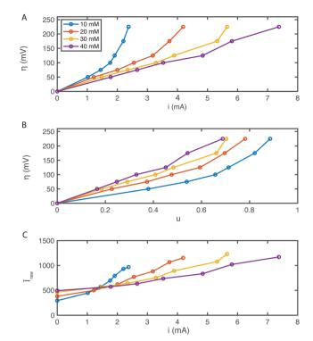
Fig. 4 Characteristic plots from MSC experiments. (A) Polarization plot as a result of the MSC experiment for [AQDS]<sub>0</sub> values indicated. (B) Applied overpotentials as function of the electrolyte utilization u. (C) Mean raw fluorescence intensity  $\bar{I}_{\rm raw}$  averaged over the entire confocal microscope image as a function of the current i.
