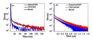
Fig. 6 Decay spectra of (a) FAPI, and (b) CsFAPI films. The black solid line is a fitting line from the bi-exponential decay function:  $I(t) = A + B_1 \mathrm{e}^{-\frac{t}{\tau_1}} + B_2 \mathrm{e}^{-\frac{t}{\tau_2}} + B_3 \mathrm{e}^{-\frac{t}{\tau_3}}.$
