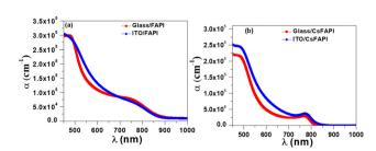
Fig. 4 The absorption coefficient of (a) FAPI and (b) CsFAPI perovskite thin films
