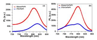
Fig. 5 Steady-state PL spectra of (a) FAPI and (b) CsFAPI thin films fabricated on different substrates
