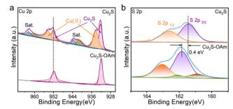
Fig. 2 High-resolution Cu 2p (a) and S 2p (b) XPS spectra of  $Cu_2S$  and  $Cu_2S$ -OAm.
