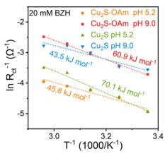
Fig. 6 Activation energies calculated from the Nyquist plot.
