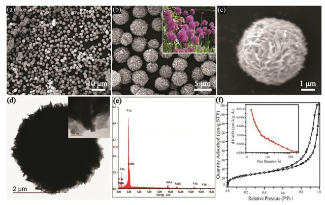
Fig. 1 SEM and TEM images of as-prepared Y-MOF samples at 120 °C for 24 h: (a) – (c) low- and high-magnification SEM images (inset in (b) is the photo of Allium giganteum);<sup>26</sup> (d) low- and high-magnification TEM images; (e) EDX spectrum;<sup>26</sup> (f) nitrogen adsorption/desorption isotherms of Y-MOFs:10%Eu3+ (inset is pore size distribution).27
