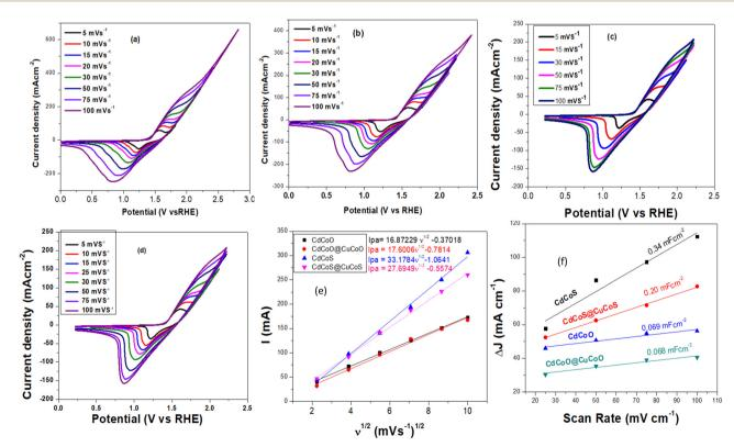
Fig. 5 Cyclic voltammograms (CV) of the catalysts (a) CdCoS, (b) CdCoS@CuCoS, (c) CdCoO, and CdCoO@CuCoO. The plots are between the anodic peak current  $(I_{pa})$  of cyclic voltammograms in 1.0 M KOH and the square root of the scan rates  $(v^{1/2})$  for all the as-synthesized catalysts.
