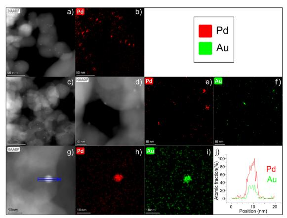
Fig. 2 (a) HAADF-STEM image of Pd/C and (b) the relative EDX of Pd distribution. (c) and (d) HAADF-STEM images of Au-Pd/C and (e) and (f) EDX analysis for Pd and Au of the region shown in f. (g) HAADF-STEM image of a single Au-Pd nanoparticle and relative EDS analysis:(h) Pd, (i) Au and (j) atomic fraction (%) profile of the selected nanoparticle.
