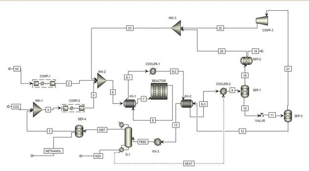
Fig. 2 Process flow for methanol production as considered in this study
