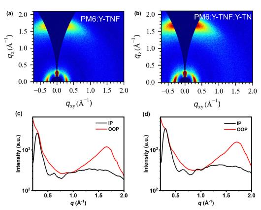
Fig. 7 (a) The two-dimensional GIWAXS patterns of PM6:Y-TNF film, (b) the two-dimensional GIWAXS patterns of PM6:Y-TNF:Y-TN film, (c) the corresponding in-plane and out-of-plane profiles under PM6:Y-TNF film optimal conditions, and (d) the corresponding in-plane and out-of-plane profiles under PM6:Y-TNF:Y-TN film optimal conditions
