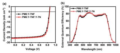
Fig. 3 (a) J-V plots of the PM6: Y-TNF: Y-TN-based OSCs (1:1:0 and 1:1:0.1, w/w/w) with 0.25% DIO additive, and a TA treatment at 100 °C for 5 min under an illumination of AM 1.5 G, 100 mW cm<sup>-2</sup>, and (b) EQE curves of the corresponding OSCs.
