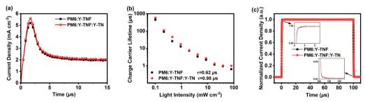
Fig. 5 (a) Photo-CELIV curves, (b) carrier lifetime curves and (c) TPC results of the binary device based on PM6:Y-TNF and the ternary device based on PM6:Y-TNF:Y-TN (1:1:0.1, w/w/w).
