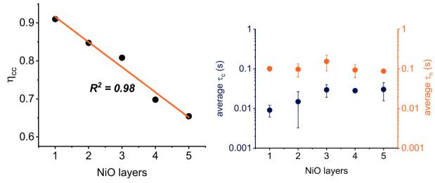
Fig. 3 Left: The charge collection efficiency  $\eta_{CC}$  versus the number of NiO layers; right: variation of the hole collection time  $\tau_c$  (navy) and hole recombination time  $\tau_n$  (orange) as a function of the number of applied NiO layers.
