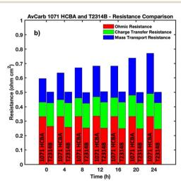
Fig. 15 (a) EIS data from the beginning and end of each experiment and (b) comparison of total resistance values of the VRFB with AvCarb 1071 HCBA and AvCarb T2314B electrodes
